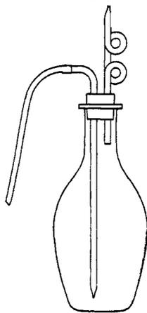
The solution to be precipitated is poured into the flask, this in turn corked up, and the apparatus stood in the hood. The gas is now passed into the solution and the flask violently shaken by hand. The bends in the exit tube keep any of the solution from being thrown out of the flask. The churning up of the solution with the hydrogen sulphide gas quickly throws out of solutions the metals of the copper-arsenic group.
